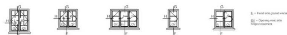
For casement windows: For exact location of each window type refer to the proposed elevations drawing: 3920 AD(0) 14.15 & 16. New and existing windows to be painted WHITE (slightly off white).
