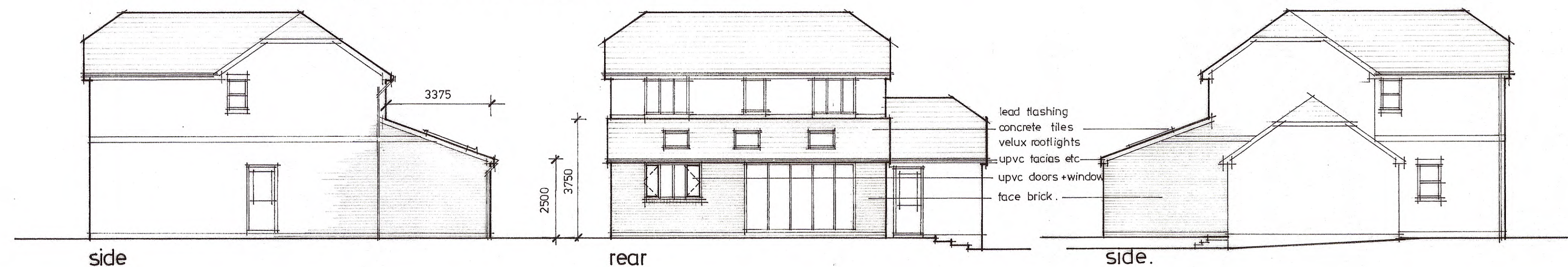
proposed elevations. 1:100. all materials of external finish and brick detailing to match existing
